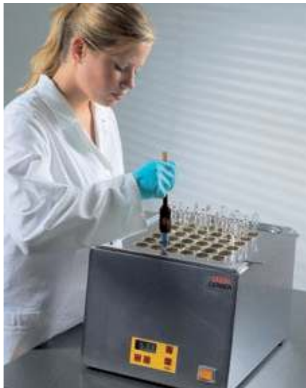
Fig. 5 The butyrometers are brought to the exact reading temperature in a water bath
