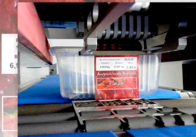
The label is applied automatically and precisely over the package edge and is pressed under the edge.
