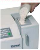
The Inframatic 9140 Flour Analyzer is a Near Infrared (NIR) spectrometer specifically designed for the analysis of flour. Its unique sample presentation system completely removes operator influence as a source of error making the Inframatic 9140 the most accurate flour analyzer available.
