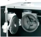
Kjeldahl etc. The Laboratory Mill 3100 is a hammer type cyclone mill, built into a soundproof casing. An adjustable vacuum feed control regulates the feed rate of the sample into a metallic grinding chamber. A hardened steel hammer rotates at high speed forcing the sample through a stainless sieve. Standard sieve of 0.8 mm is used for Falling Number, Glutomatic System and NIR analyses. Sieves from 0.5 - 2.0 mm are available. The fine, homogeneous sample is separated from air in a cyclone and
