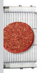
Usable mold plate area 6" (152mm) wide by 6" (152mm) front to back
