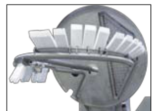
Inclined, removable scraper arm and satellite mixer.
