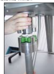
Inclined, removable scraper arm and satellite mixer.
